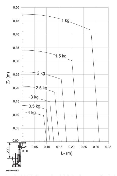
Extra load of 10 kg (hose package included) at the upper arm housing included in the load diagram.
