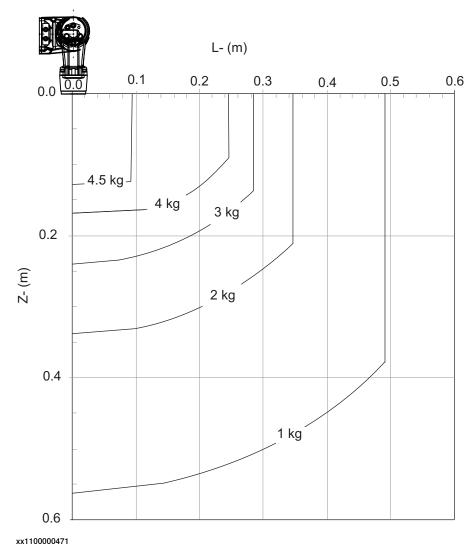
Extra load of 10 kg (hose package included) at the upper arm housing included in the load diagram.
