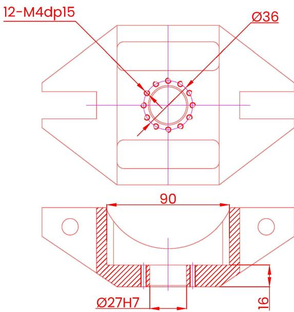
基座安装 Base installation (mm)
