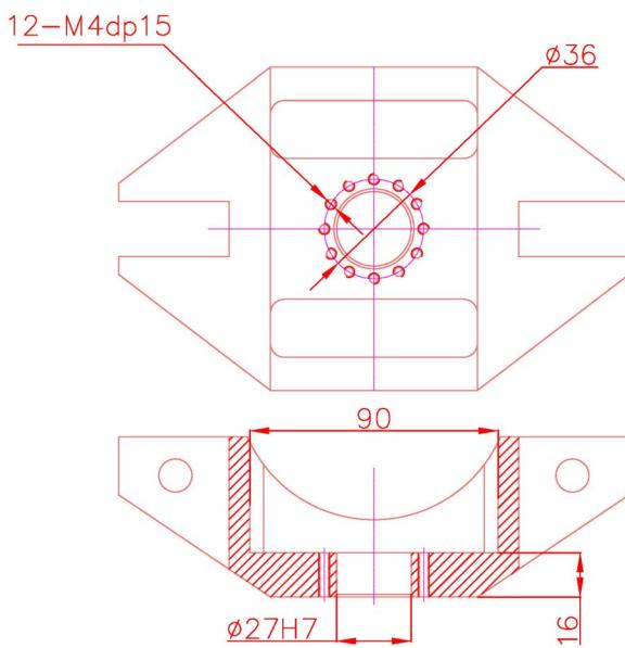
基座安装 Base installation (mm)
