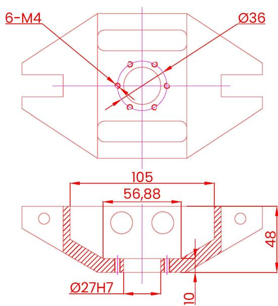
基座安装 Base installation (mm)
